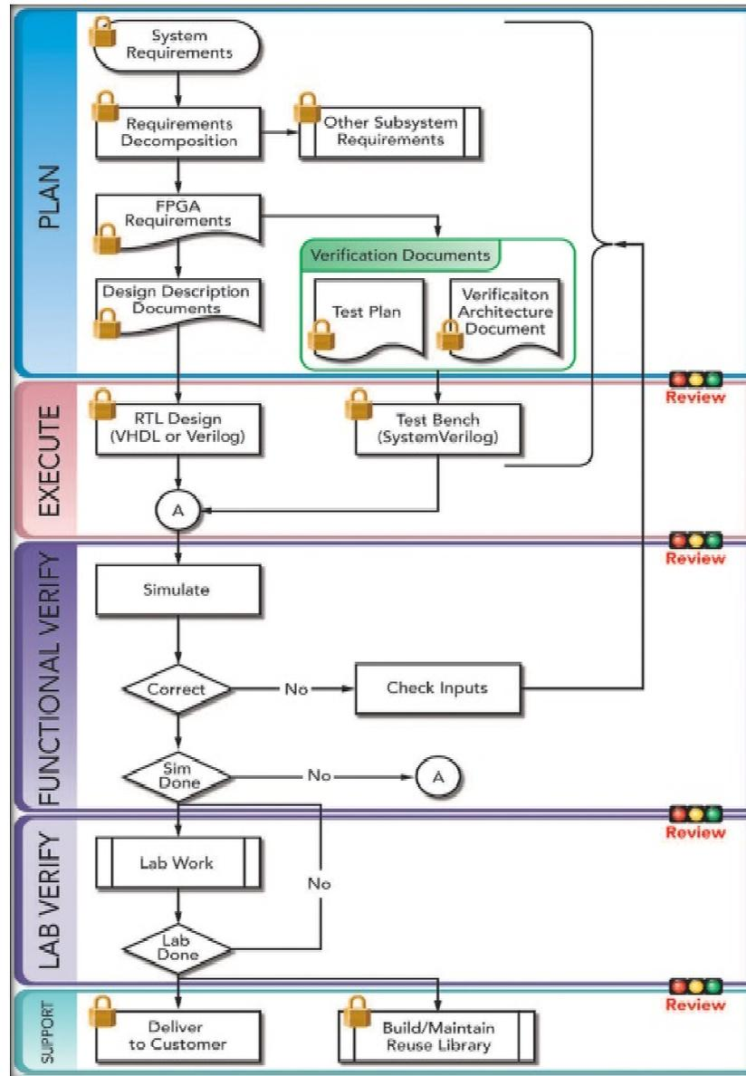
Figure 2. Typical Best Practice Electronic Design Process [11]
