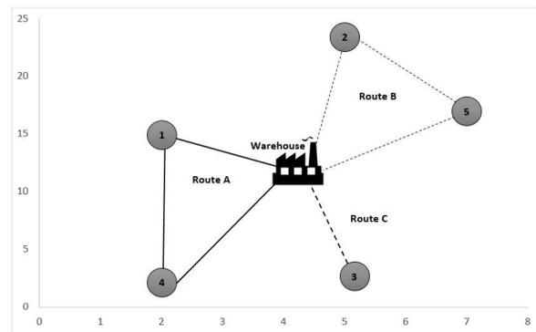
Figure 3 shows when the vehicle capacity is less compared to Figure 2, which is 30 tons. The vehicle needs to serve five retailers, but the inventory carried is not enough. In that case, the route has to extend to become three routes in order to fulfil the requirements. The vehicle has to take route A  $= (0-1-4-0)$ , route B  $= (0-2-5-0)$ , and route C  $= (0-3-0)$ .
