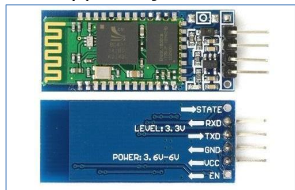
Figure 4. Bluetooth HC-06 Module
