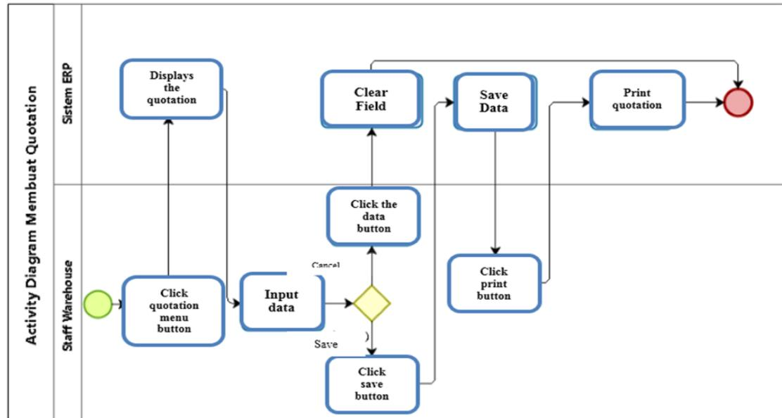
**Figure 6.** Activity Diagram Making Quotation
